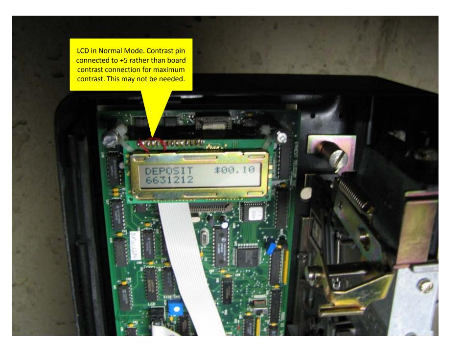
The following slides show the configuration of my pay phone for use on my Asterisk PBX via an ATA. I am using the 7 digit and 10 digit rate override settings to override the built-in rate table, which can't be easily changed.
